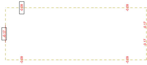
M 1 : 128 Sector of system Group 0 Bending moment m_{xx} in local x in Nodes ↕, Loadcase 2 ΥΔΡΟΣΤΑΤΙΚΗ→ΠΛΗΡΗΣ, from -0.172 to 0 step 5.00 kNm/m
